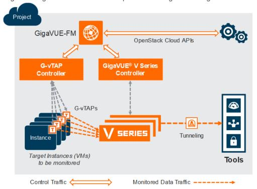
A G-vTAP agent is deployed by installing the agent in the virtual instances. When a G-vTAP agent is installed, a G-vTAP Controller must be configured in your environment. A G-vTAP Controller orchestrates the flow of mirrored traffic from G-vTAP agents to the GigaVUE Cloud Suite V Series nodes. A single G-vTAP Controller can manage up to 100 G-vTAP agents deployed in the cloud.
